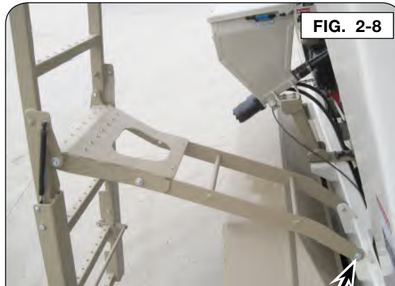
Secure ladder with 3/8"-16UNC locknut, 3/8" SAE flat washer (9405-086), nylon bushing (2003029), and 3/8"-16UNC x 1 1/4" capscrews (9390-056).
